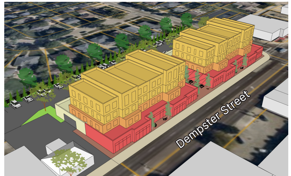
Figure 2.12: An overlay district can include design standards for proposed development including materials, fenestration, streetscape environment and landscape buffers
