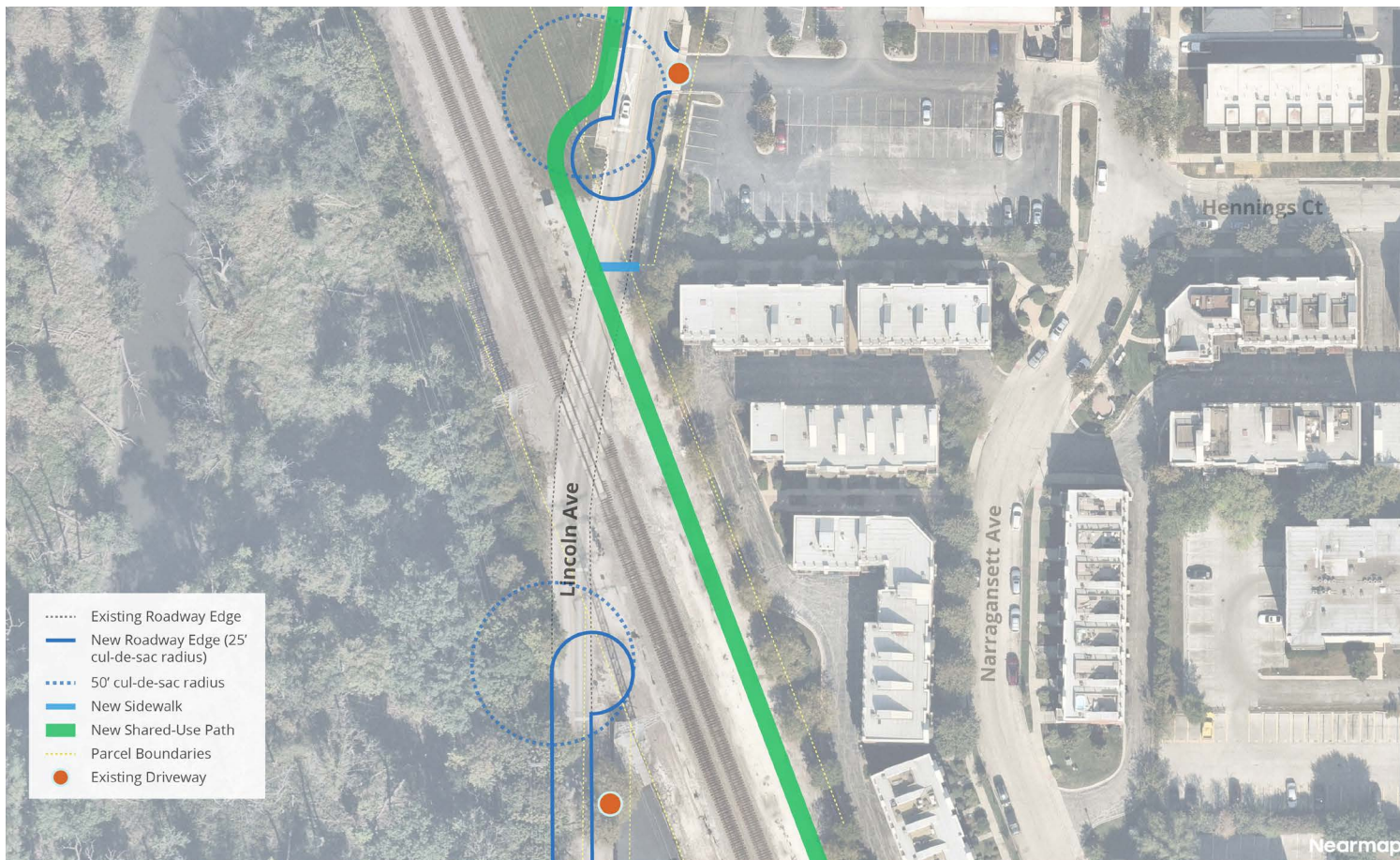
Figure 2.22: Lincoln Avenue Railroad Crossing Closure
