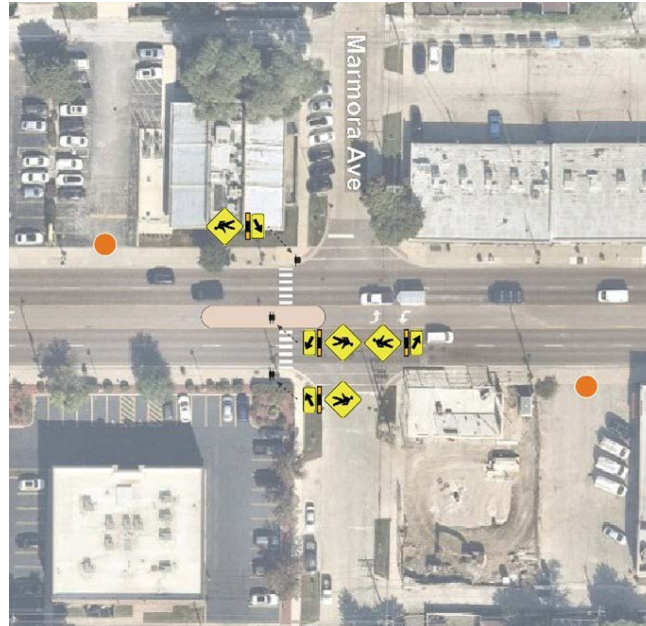
Figure 2.17: Marmora Avenue New Crossing
