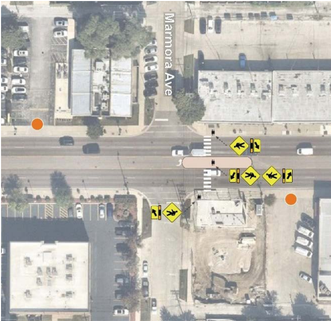
Figure 2.16: Marmora Avenue New Crossing
